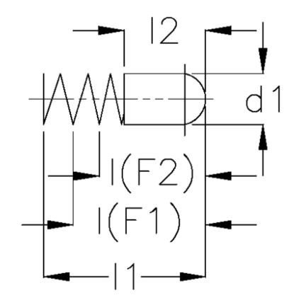
$\begin{array}{lll} \text{d1} & = 5.0 \\ \text{I(F1)} & = 13.0 \\ \text{I(F2)} & = 10.4 \\ \text{I1} & = 16 \\ \text{I2} & = 8.0 \\ \text{Spring pressure (F1) N} = 8.0 \\ \text{Spring pressure (F2) N} = 15.0 \end{array}$
